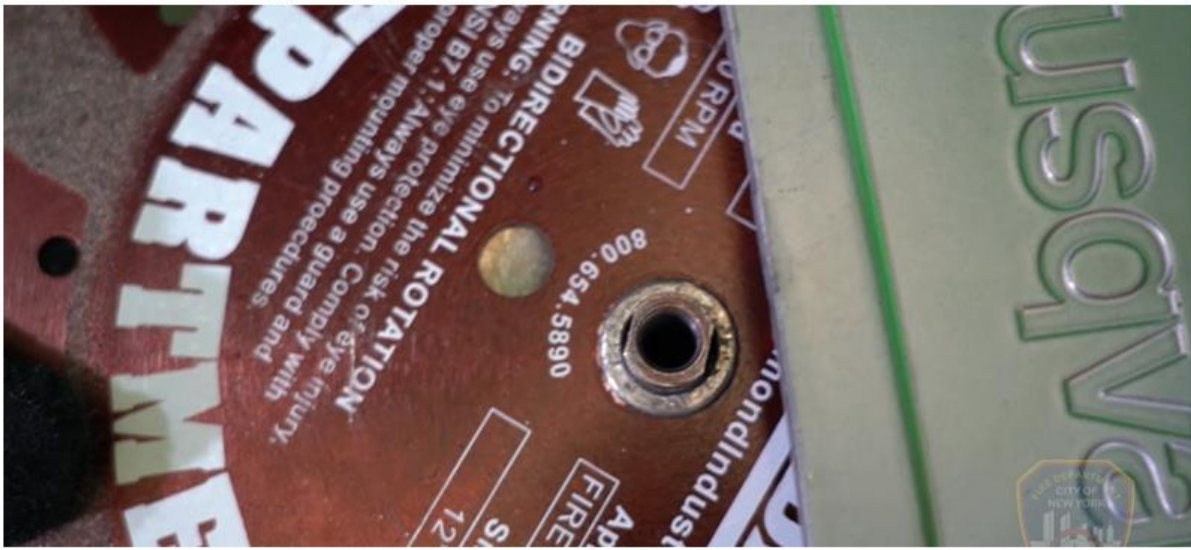
The inner bore of the blade must align with the flange properly - as pictured above
